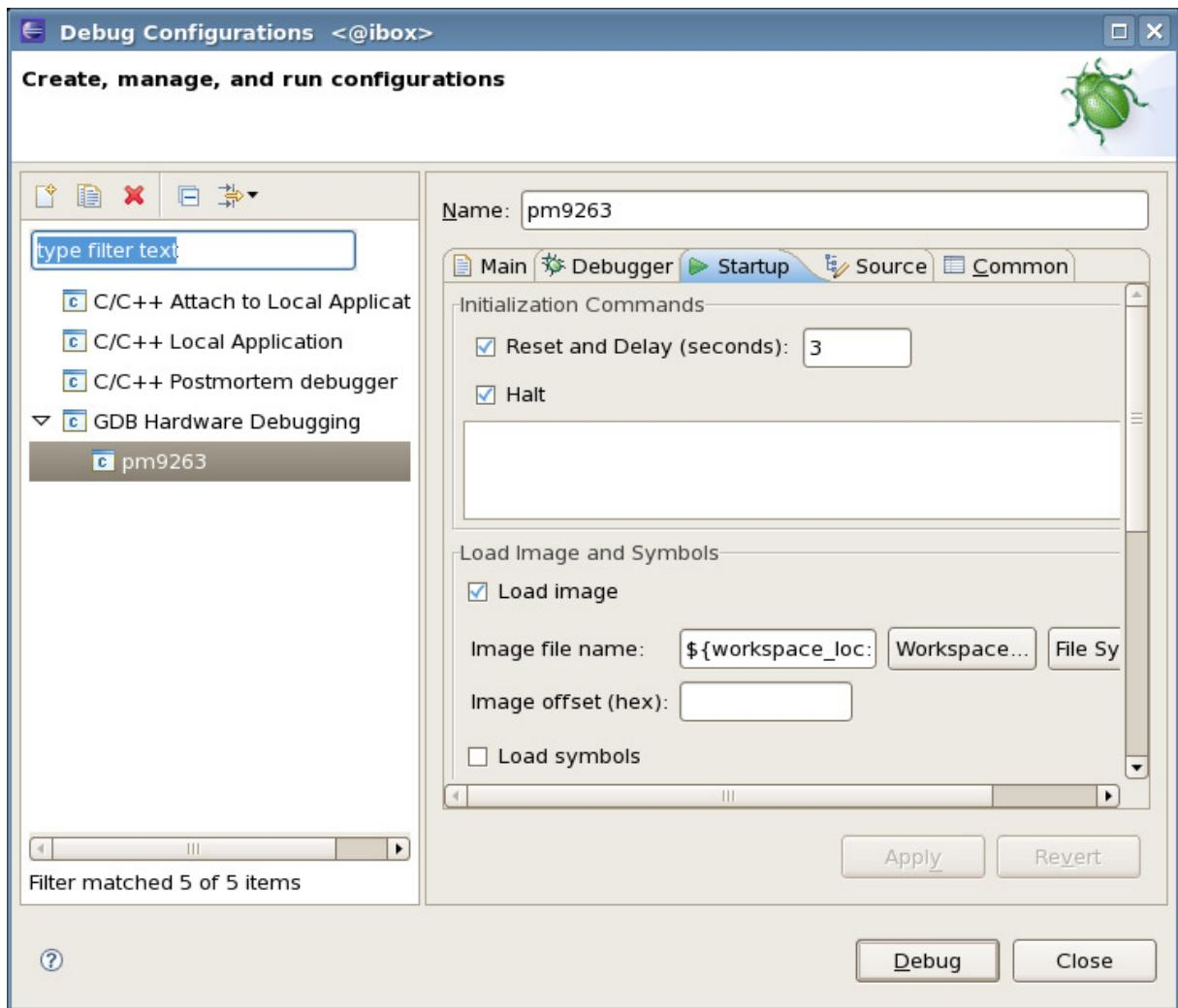
Now click on the “Debug” button and the Eclipse debugger will start. You should also change to debug perspective. To start the application just type in the console window: “c”.
